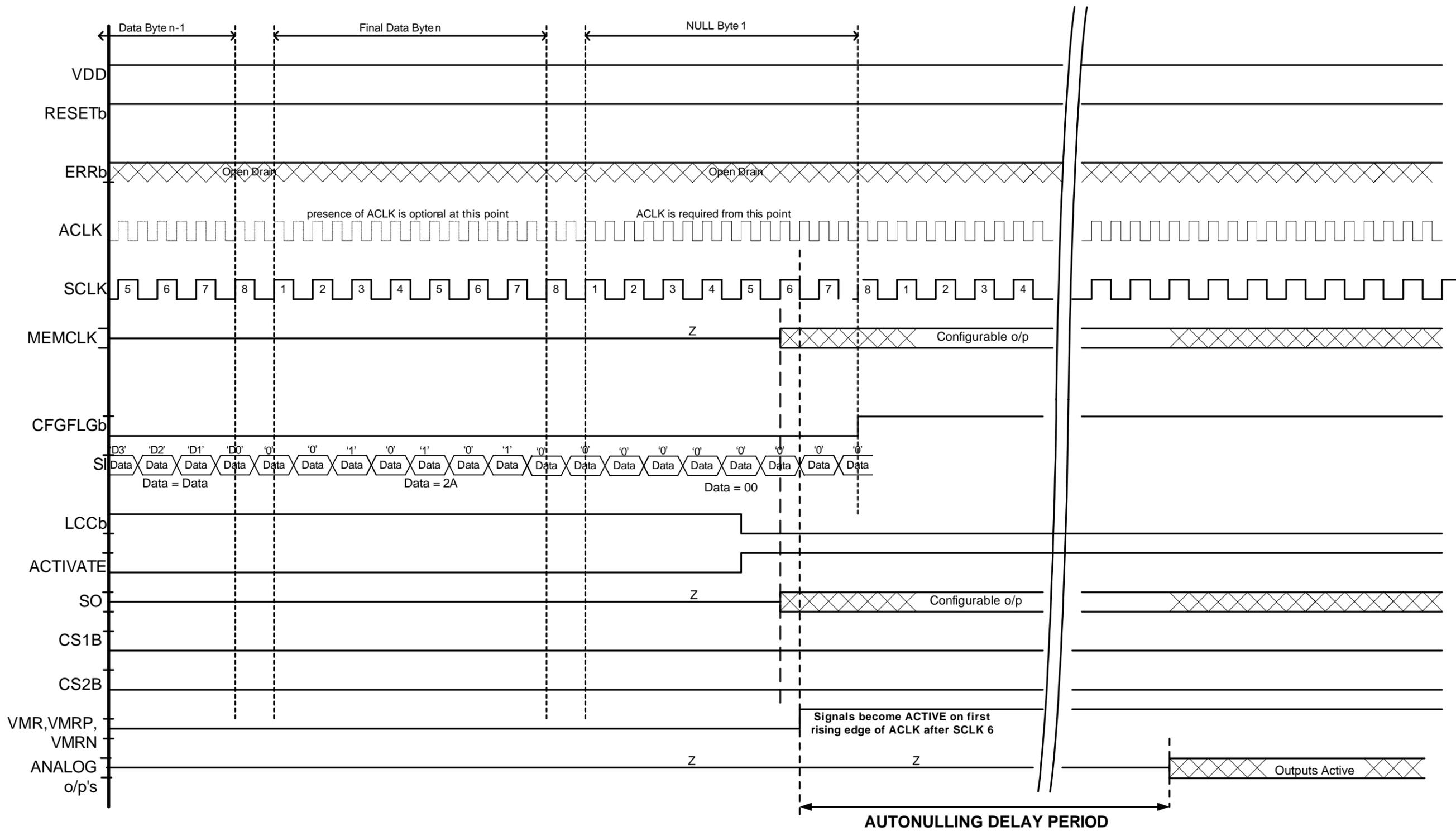
IF AUTONULLING is not used, then the Autonulling delay period is Zero.
